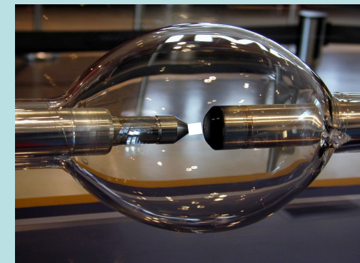
15 kW Xenon arc lamp
